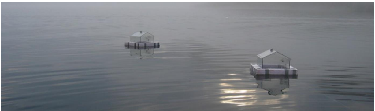
Systems for sampling gases released from lake surfaces (photo, SINTEF Ocean)
