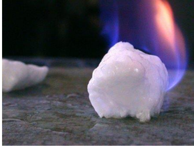
A flammable gas hydrate (U.S. Department of Energy, Office of Fossil Energy and Carbon Management).
